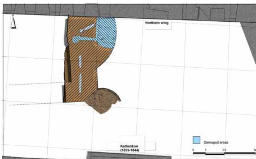
Drawing 1. St Paul's monastery; ground plan drawing of the revealed remnants (scale 1:50)
