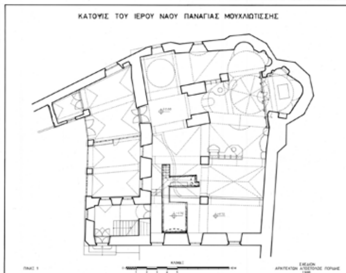
Fig. 2. Church plan showing the underground space.
