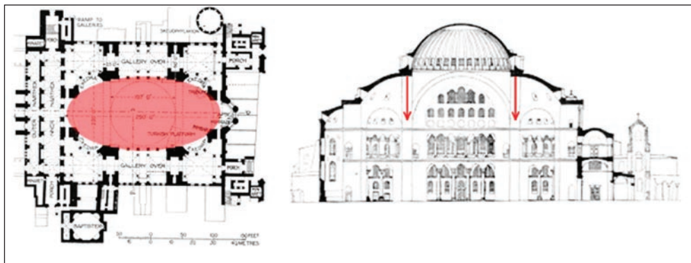
Fig. 2 Ground plan and longitudinal cross-section of the church Hagia Sophia
